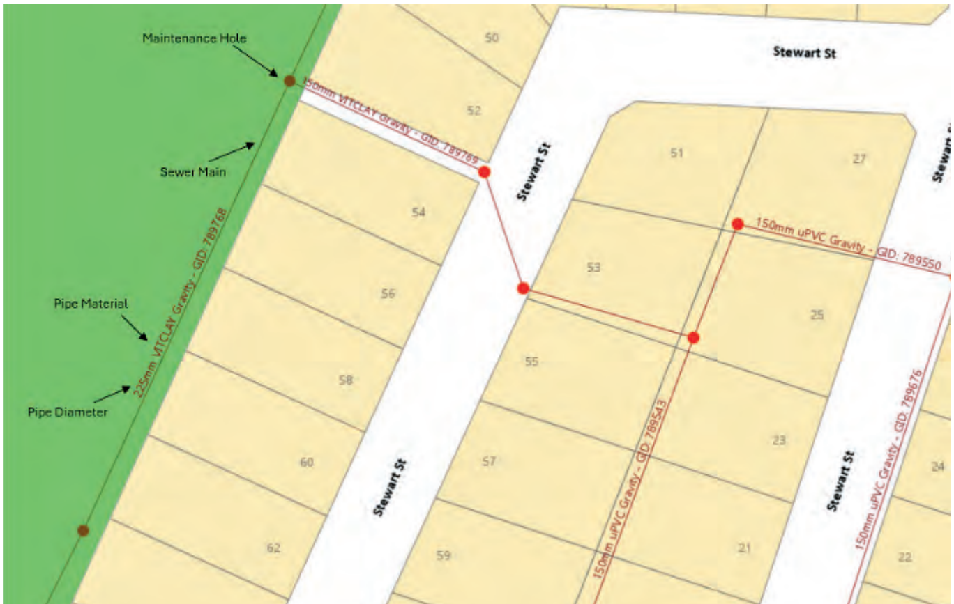
Figure 4: Sewer asset plan
