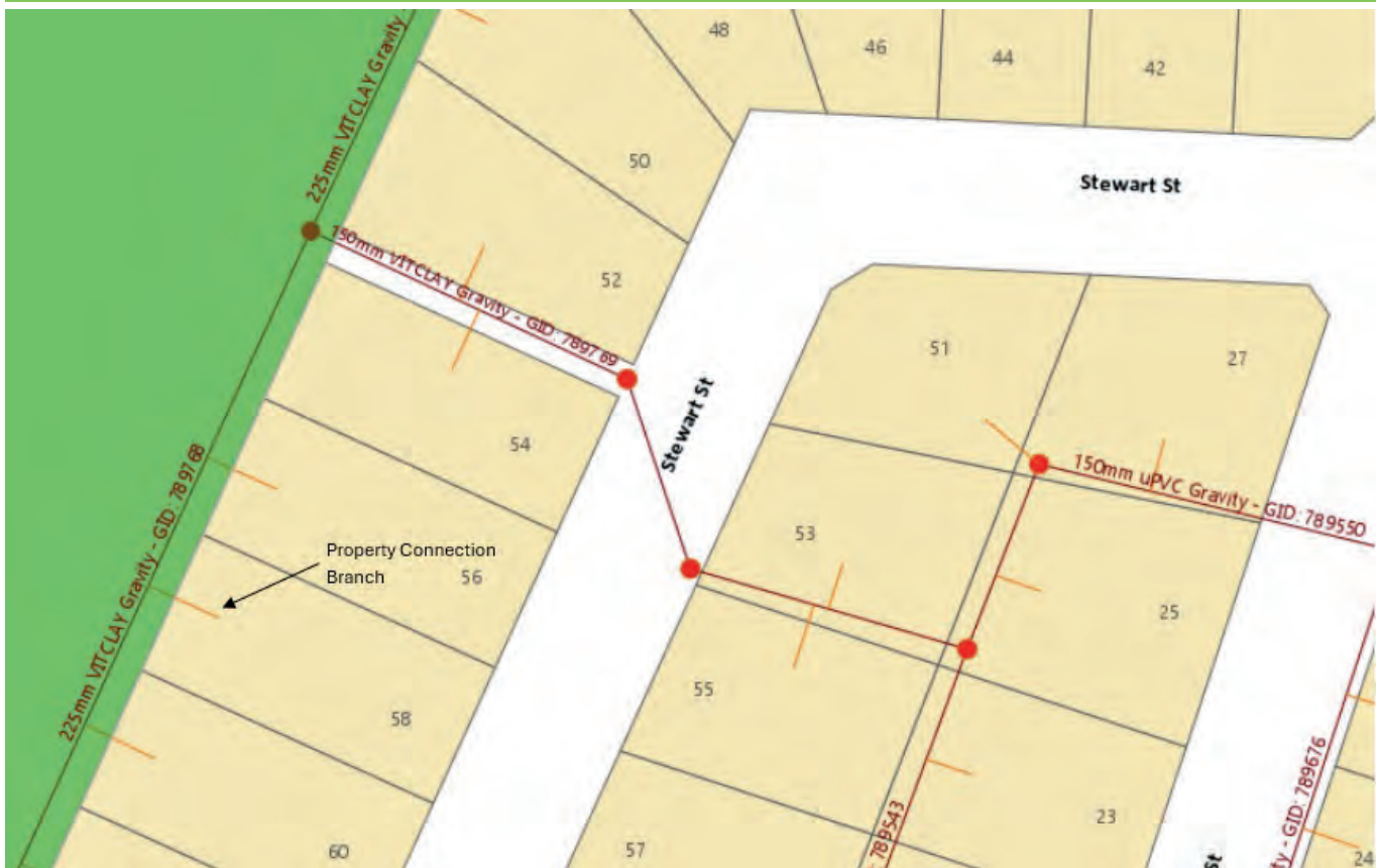
Figure 10: Sewer connection branch-asset plan
